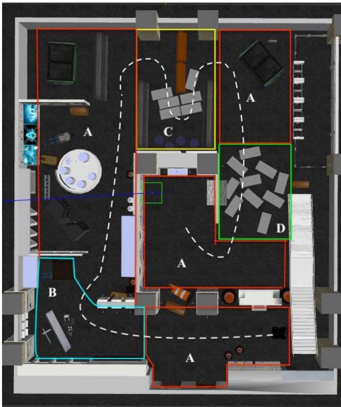
Fig. 2. The tessellations (A to D) and the feasible robot path plan P (dotted line) for the navigation task
