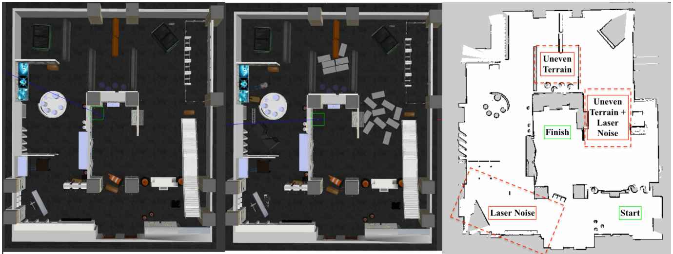
Fig. 3. Navigation Task Arena (L to R): 1) Empty, 2) With obstacles and uneven terrain, 3) 2D map with start and finish points marked, and locations where performance degradation is introduced.
