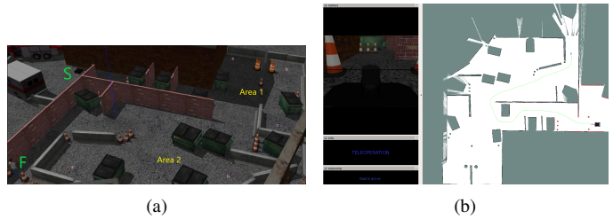
Fig. 3. 3(a) : The arena used in the experimental evaluation, simulating a disaster response scenario. 3(b) : The Graphical User Interface (GUI). Left : Video feed from the camera, the control mode in use and the state of the robot. Right : The map (as created by SLAM) showing the position of the robot, the current goal (blue arrow), the AI planned path (green line).
